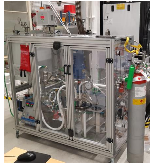
Methanation test unit "MoMe"
